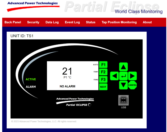
Browser-Based Graphical User Interface For Monitoring, Alarms, Settings, File Transfer, and Data Log
